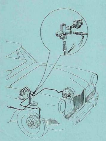
Instances have been reported of the brake pipe Part No. 11H215 positioned between the five way connection and L/H front brake hose lying too close to the rear of the engine. Also the brake pipe Part No. 1H5717 laying too close to the starter motor and gearbox mounting plate.
