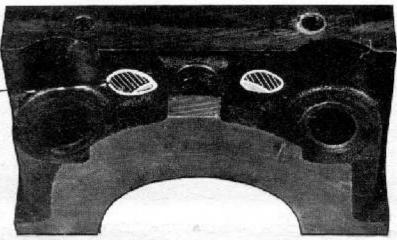
The utmost care must be taken during assembly to ensure complete cleanliness and the correct fitting of all bearing shells with tangs properly located in their slots. Care should also be taken when fitting the rear main bearing cap, to ensure that the rear face is flush with the back of the engine block, by tapping slightly as necessary.
